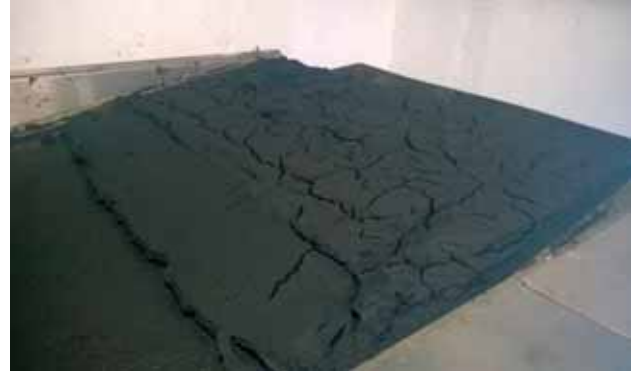
Picture 5: After the separation of the water the sludge is very dry
