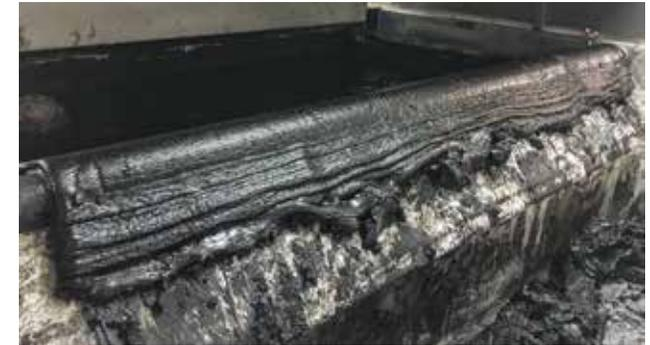
During the water treatment process practically all water is separated from the residues and therefore the waste that need to be disposed of is highly concentrated - bringing savings in waste disposal costs. Here pictured a sample of waste showing the solid consistence of it.
